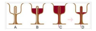
Cross section of a Pythagorean cup being filled: at B, it is possible to drink all the liquid in the cup; but at C, the siphon effect causes the cup to drain
